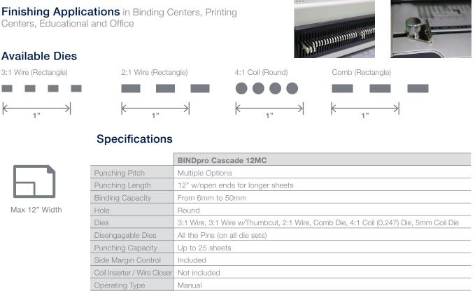
Operating TypeManualWeightMachine: 24lbs (10.9kgs) Die: 18lbs (8.2kgs)Warranty1 Year Parts Warranty, not including wearable parts
